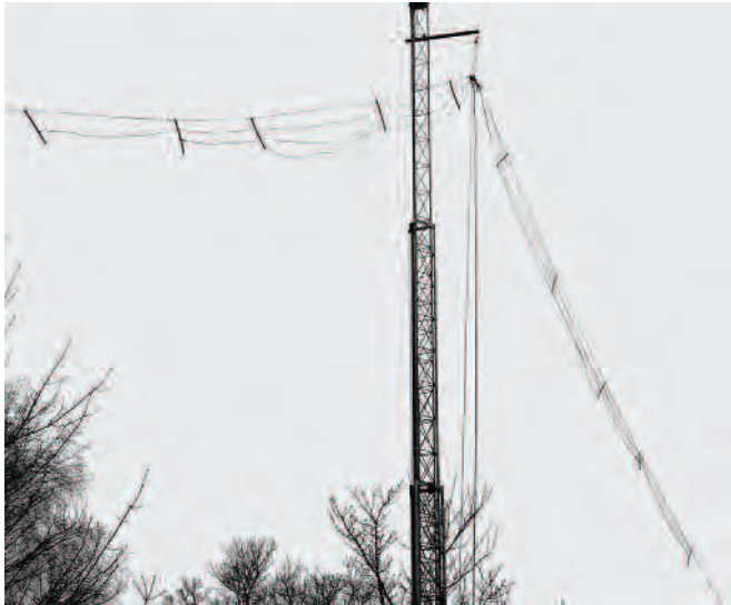
PHOTO 1: A practical installation of a multiband dipole constructed from drop feed telephone wire and plastic high pressure water pipe as spacing insulators. The spacing between each of the elements should be about 6cm (just over 2in).
