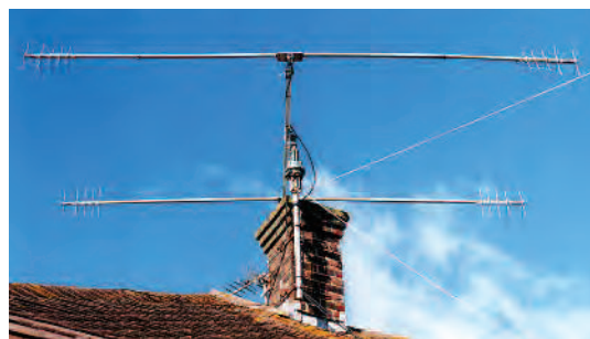
PHOTO 3: The antenna in Photo 2 rebuilt by extending the elements and boom and modifying the element end resonators.
